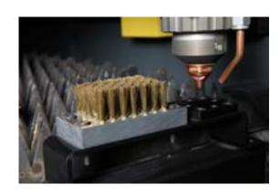
CNC controlled feature allows cleaning and quick calibration of nozzle at predefined numbers of piercing. Applying auto nozzle cleaning avoids problems caused by stacked spatters and ensure height following accuracy.
